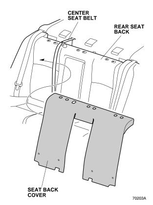
Secure the three hook-and-loop fasteners to the rear seat back. Raise the rear seat back and lock it to its original position.
