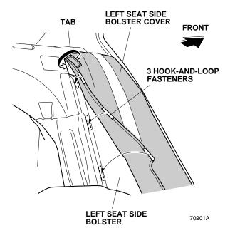
7. Insert the two tabs to the left seat side bolster.
