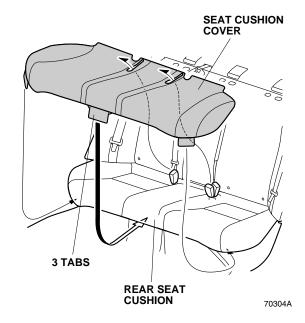
17. Insert the seat cushion cover between the rear seat back and the rear seat cushion, and secure the three hook-and-loop fasteners to the rear seat cushion.
