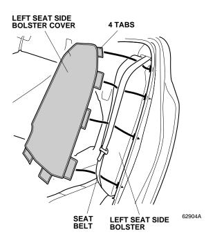
Insert the tab on the left seat side bolster cover to the left seat side bolster. Secure the three hook-andloop fasteners to the left seat side bolster.
