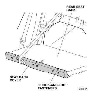
Insert the seat back cover under the headrest guides. Pull down the armrest, secure the hook-andloop fastener to the rear seat back.
