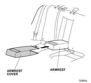
Raise the armrest. Pull out the armrest cover between the armrest and rear seat back, and secure the hook-and-loop fasteners on the armrest cover as shown.
