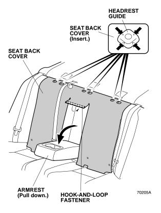
12. Insert the seat back cover between the rear seat back and the rear seat cushion, secure the four hook-and-loop fasteners to the rear seat back.
