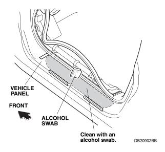
Align the left front illuminated door sill trim with the masking tapes and install the left front door sill trim to the vehicle panel.
