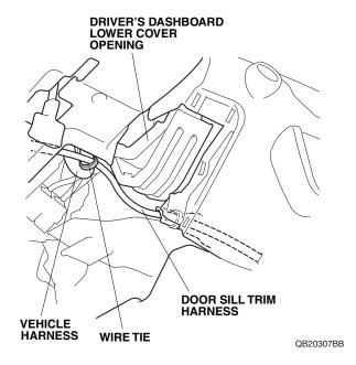
63. On the passenger's side of the vehicle, route the door sill trim harness and secure it to the vehicle harness with two wire ties.
