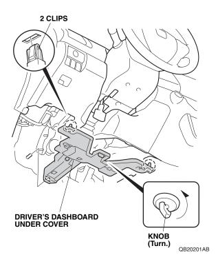
6. Remove the driver's dashboard lower cover (nine clips and unplug the vehicle connectors).
