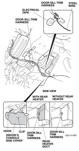
58. Attach a piece of steel wire to the door sill trim harness with electrical tape. Route the door sill trim harness through the center console from the driver's dashboard lower cover opening to the passenger's under cover opening.
