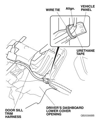
Secure the door sill trim harness to the vehicle harness with one wire tie. Move the steering wheel up and down through its full adjustment range and make sure the door sill trim harness is not being stretched.
