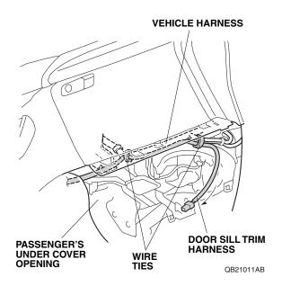
64. Route the door sill trim harness and secure it to the vehicle panel and vehicle harness with two wire ties.
