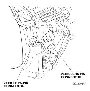
44. Plug the vehicle 25-pin connector into the door sill trim harness 25-pin connector. Plug the door sill trim harness 25-pin connector into the vehicle 25-pin connector.
