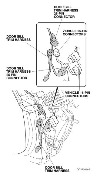
45. Re-plug the vehicle 16-pin connector.
