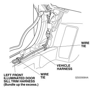
52. Bundle up the excess left front illuminated door sill trim harness, and secure it to the vehicle harness with one wire tie.
