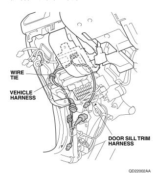
43. Unplug the vehicle 16-pin connector and 25-pin connector.
