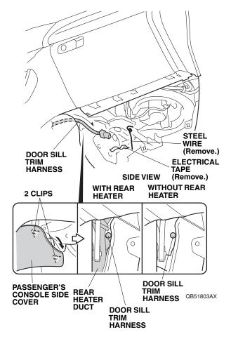
60. Route the door sill trim harness, and remove the electrical tape and steel wire.
