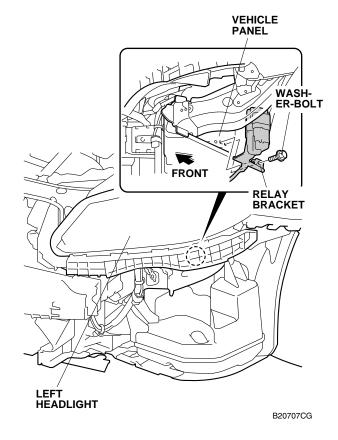
24. Route the fog light harness as shown. Remove the vehicle ground bolt, and secure the fog light harness ground terminals A and B to the vehicle ground terminal. Reinstall the vehicle ground bolt.
