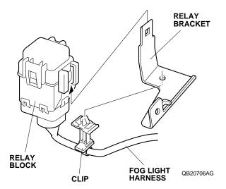
22. Secure the clip from the fog light harness to the relay bracket.
