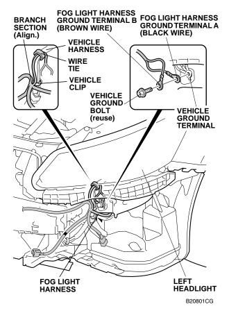
25. Secure the fog light harness to the vehicle harness with one wire tie at the location shown.
