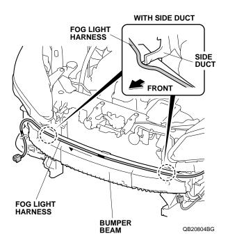
30. Align the green tape on the fog light harness with the vehicle clip, and secure the fog light harness to the vehicle harness with one wire tie.
