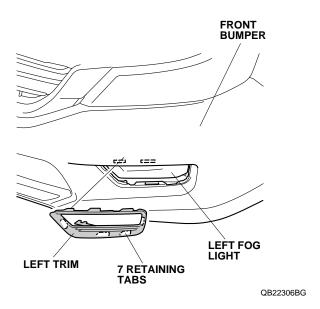
3. Remove the fog light (two self-tapping screws, two retaining tabs and unplug the vehicle connector).
