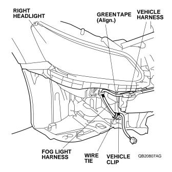
35. With the help of an assistant, bring the front bumper close to the vehicle. Plug the two fog light harness 2pin connectors into the left fog light subcord 2-pin connector and right fog light, and reinstall the front bumper.
