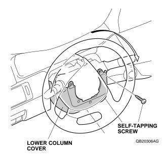
7. Remove the lower column cover (one self-tapping screw).
