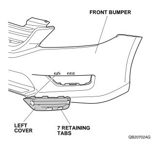
16. Install the left trim to the front bumper with seven retaining tabs.
