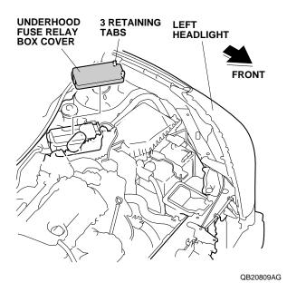
37. Plug the 15A fuse into the underhood fuse relay box.
