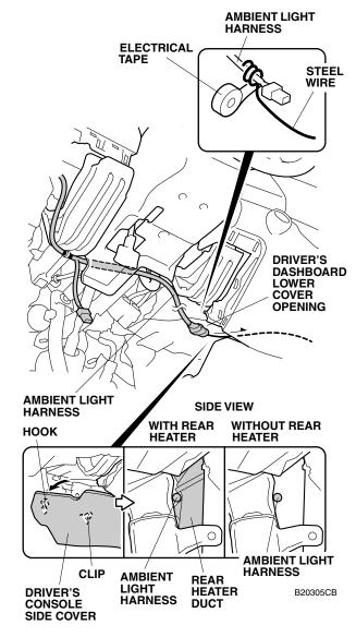
14. Attach a piece of steel wire to the ambient light harness with electrical tape. Route the ambient light harness through the center console from the driver's dashboard lower cover opening to the passenger's under cover opening.
