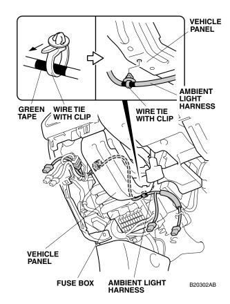
Using diagonal cutters, cut the clip portion off of one wire tie.
