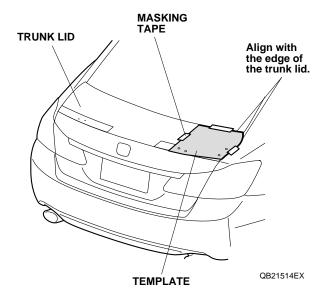
14. Using a felt-tip pen, mark the trunk lid through the hole in the template. Remove the template.
