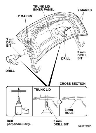
To prevent the metal shavings from falling into the trunk floor area, attach tape over the each hole as shown.
