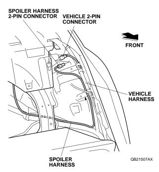
57. Plug the spoiler harness 2-pin connector to the vehicle 2-pin connector.
