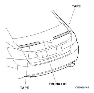
11. Place the template on the trunk, and align it with the left edge of the trunk lid. Tape the template to the trunk lid with masking tape.
