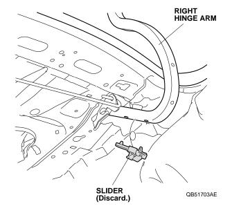
44. Remove and discard the two holders from the hinge bracket.
