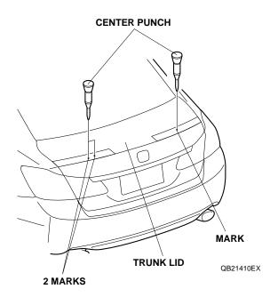
While wearing eye protection, drill two marks with a 8 mm hole cutter. Drill perpendicularly to the trunk lid.
