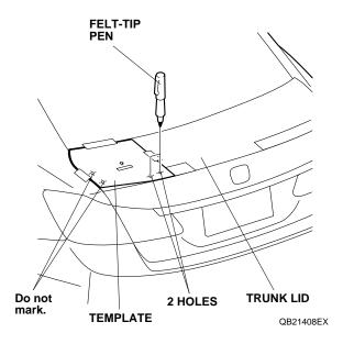
13. Turn the template over and install it on the right side of the trunk the same way.
