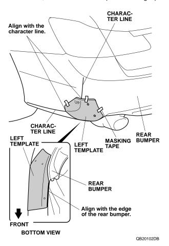
Using a pushpin, pierce the rear bumper through the three holes in left template. Remove the left template.
