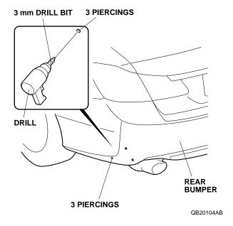
5. Enlarge the two upper holes to 12 mm using a 12 mm drill bit. Remove any burrs.
