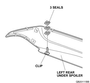
13. Using one alcohol swab, thoroughly clean the rear bumper where the left rear under spoiler will attach.
