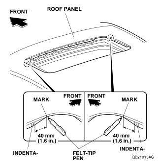
4. Using isopropyl alcohol on a shop towel, clean the roof area and the inside edge of the moonroof opening. Starting at the mark you made, clean about 2 inches toward the front of the opening but don't wipe off the mark.
