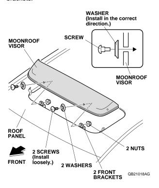
Loosely install the moonroof visor to the side brackets with two screws, two washers, and two nuts. Remove the masking tape from the side brackets.
