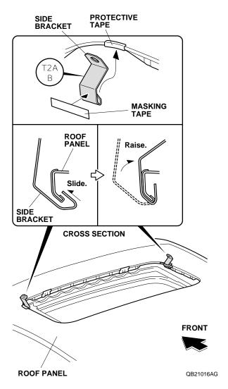
12. Place one front bracket into position over the protective tape, and align the lower portion of the front bracket with the indentation in the roof panel. Tape it into position with masking tape.
