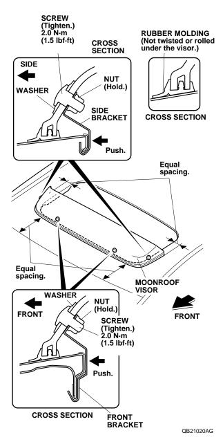
17. Tighten the two screws on the side of the opening first, then tighten the two screws on the front. Apply pressure so that there is no gap between the brackets and the roof panel. Torque the screws to 2.0 N·m (1.5 lbf·ft).
