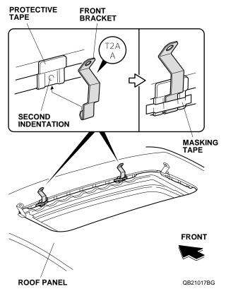
13. Install and tape the other front bracket to the moonroof opening the same way.
