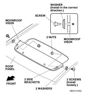
Position the moonroof visor with equal spacing in the front and on the sides. Check that the rubber molding is not twisted or rolled under the visor.
