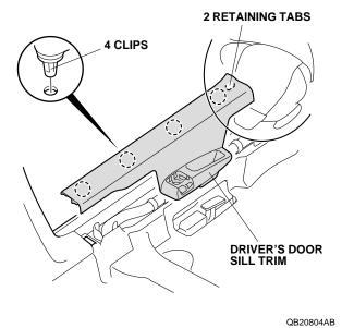
2-Door: Two retaining tabs and six clips.
