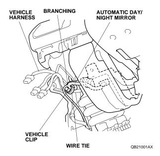
29. Route the automatic day/night mirror harness ground terminal toward the vehicle ground terminal.
