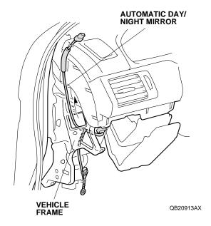
28. Secure the automatic day/night mirror harness to the vehicle harness with one wire tie as shown.
