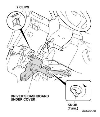
Remove the driver's dashboard lower cover (nine clips and unplug the vehicle connectors, if equipped).
