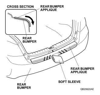
14. Using a shop towel, wipe up the 3M protective tape application solution. Allow the rear bumper applique to dry thoroughly. Remove the masking tape.
