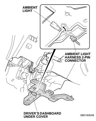
Plug the ambient light harness 2-pin connector into the ambient light, and reinstall the driver's dashboard under cover.
