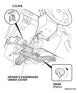
4. Remove the driver's dashboard lower cover (nine clips and unplug the vehicle connectors).
