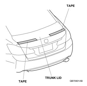
Place the template on the trunk, and align it with the left edge of the trunk lid. Tape the template to the trunk lid with masking tape.
