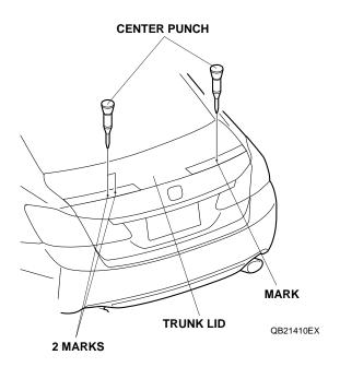
While wearing eye protection, drill two marks with a 8 mm hole cutter. Drill perpendicularly to the trunk lid.
