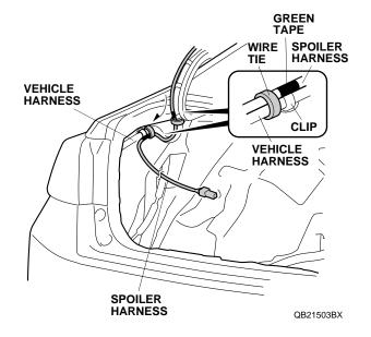
53. Secure the spoiler harness to the vehicle harness with five additional wire ties as shown.
