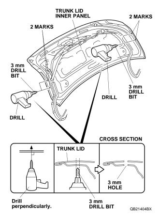
To prevent the metal shavings from falling into the trunk floor area, attach tape over the each hole as shown.
