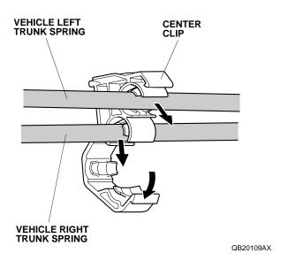
42. With an assistant holding the trunk lid open, remove the old right trunk spring from the slider using the trunk spring tool. Wear gloves to protect your hands, and push the trunk spring tool slowly and carefully.
