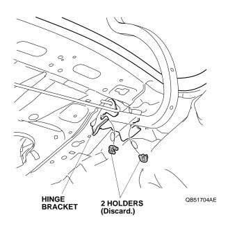
45. Install the new holders to the hinge bracket. Make sure the holders are installed in the correct orientation.
