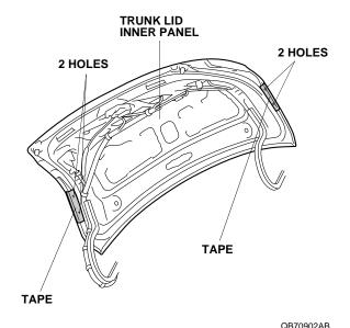
22. Enlarge the four holes made in the trunk lid inner panel in step 20 with a 11 mm hole cutter. Do not drill through the outer skin. Drill perpendicularly to the trunk lid.
