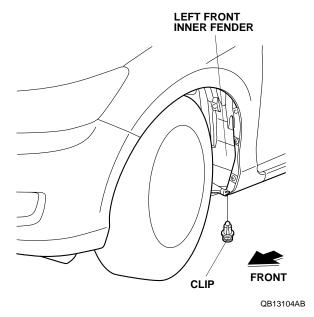
Install the left front splash guard to the left front inner fender with two washer-screws and the clip removed in step 3. Install the screws in this order
