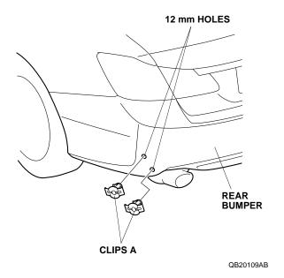
8. Using a pushpin, pierce the rear bumper at the dimple on the rear fenderwell.
