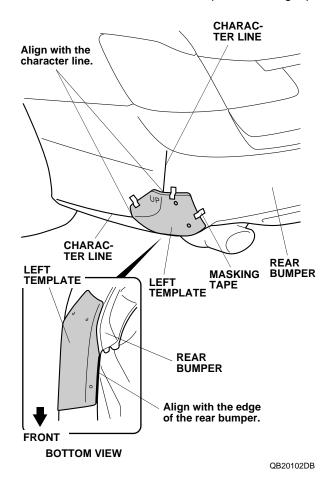
Using a pushpin, pierce the rear bumper through the three holes in left template. Remove the left template.
