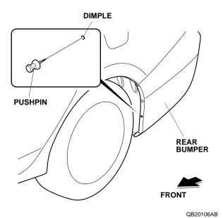
Thread a self-tapping screw into the pierced mark to make a hole in the rear bumper. Remove the selftapping screw.
