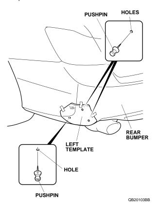
4. While wearing eye protection, drill the three piercings in the rear bumper with a 3 mm drill bit.
