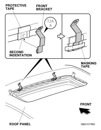
Install and tape the other front bracket to the moonroof opening the same way.
