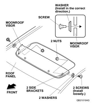
Position the moonroof visor with equal spacing in the front and on the sides. Check that the rubber molding is not twisted or rolled under the visor.
