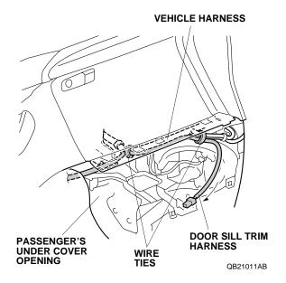
60. Route the door sill trim harness and secure it to the vehicle panel and vehicle harness with two wire ties.
