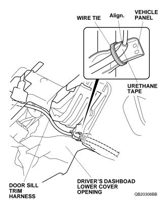
58. Secure the door sill trim harness to the vehicle harness with one wire tie. Move the steering wheel up and down through its full adjustment range and make sure the door sill trim harness is not being stretched.
