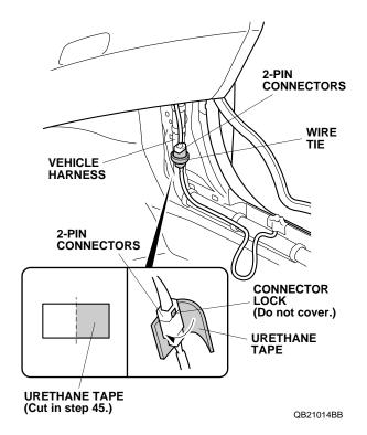
Secure the 2-pin connectors to the vehicle harness with one wire tie.
