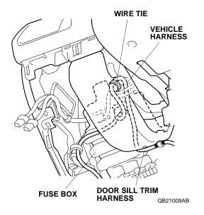
53. Release the driver's console side cover (one hook and one clip).
