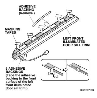
19. Using one alcohol swab, thoroughly clean the vehicle panel where the left front illuminated door sill trim will attach.
