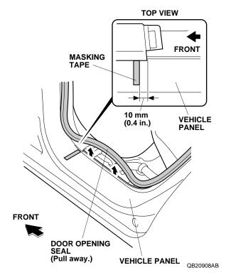
30. Attach a piece of masking tape to the vehicle panel in the location shown.
