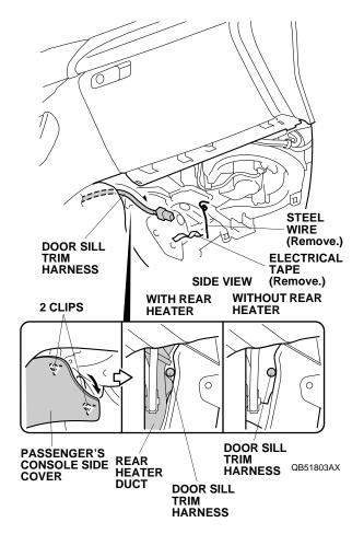
56. Route the door sill trim harness, and remove the electrical tape and steel wire.
