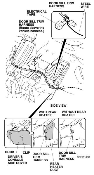
54. Attach a piece of steel wire to the door sill trim harness with electrical tape. Route the door sill trim harness through the center console from the driver's dashboard lower cover opening to the passenger's under cover opening.
