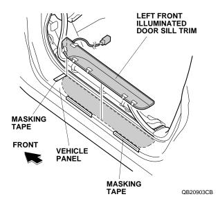
21. While applying light pressure against the left front illuminated door sill trim, carefully remove the adhesive backings.
