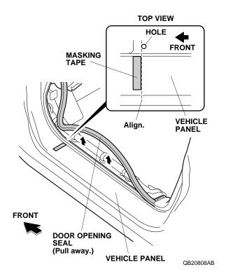
15. Attach a piece of masking tape to the vehicle panel in the location shown.
