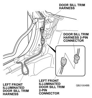
44. Plug the left front illuminated door sill trim harness 2-pin connector into the door sill trim harness 2-pin connector.
