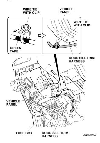
50. Using diagonal cutters, cut the clip portion off of one wire tie.
