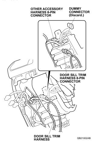
42. Route the door sill trim harness as shown, and secure the door sill trim harness to the vehicle harness with two wire ties.
