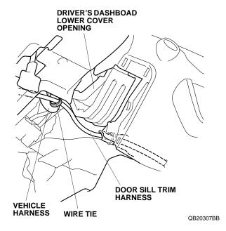
59. On the passenger's side of the vehicle, route the door sill trim harness and secure it to the vehicle harness with two wire ties.
