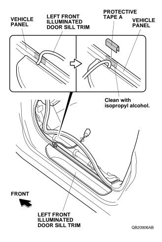
25. Install the protective clip to the protective tape A on the vehicle panel.
