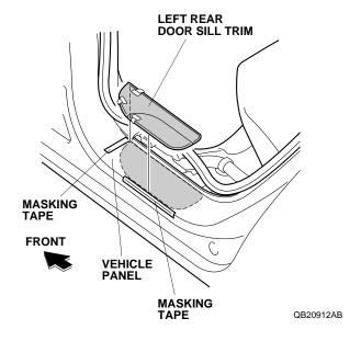
While applying light pressure against the left rear door sill trim, carefully remove the adhesive backings.
