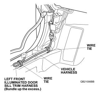
48. Secure the left front illuminated door sill trim harness to the vehicle harness with one wire tie.
