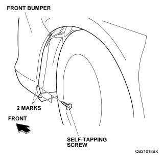
8. Install one spring nut over each hole in the front bumper in the direction shown.
