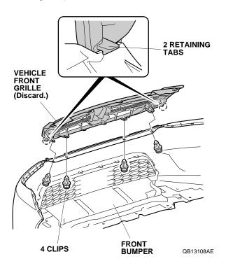
5. Install the front grille to the front bumper with the four clips removed in step 4 and two retaining tabs.
