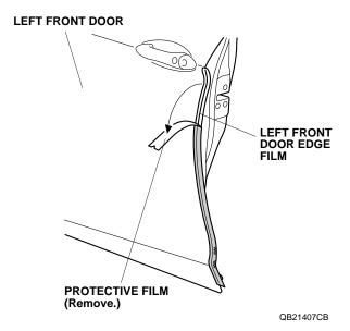
Starting from the center and working outward, use your finger to fold the left front door edge film inside the left front door. Move the your finger in one direction only. Do not damage the door seam sealant.
