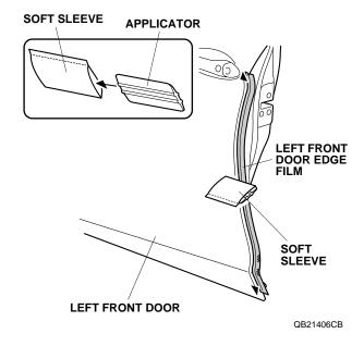
9. Slowly remove the protective film from the left front door edge film.
