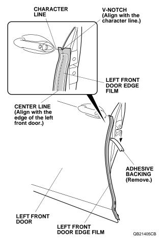
7. Align the center line on the left front door edge film with the edge of the left front door. While applying light pressure, carefully remove the adhesive backing.
