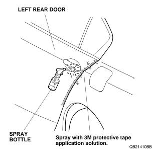
13. Open the left rear door. Peel back about 50 mm (2.0 in.) of adhesive backing from the left rear door edge film. Align the V-notch on the left rear door edge film with the left rear door as shown.
