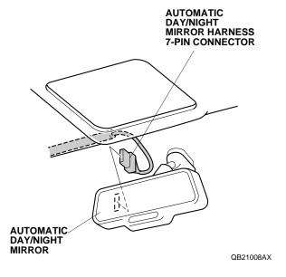
37. Install the automatic day/night mirror harness into the groove in the harness cover. Secure the harness cover to the mirror stay. Slide the harness cover behind the headliner.
