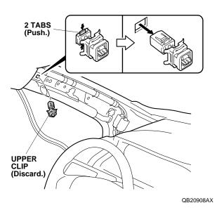
14. Install the new clip (supplied) to the driver's A-pillar trim, but do not reinstall the trim at this time.
