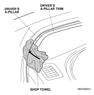
12. Slide the driver's A-pillar trim up to remove it from the upper clip. Carefully remove the shop towel and any clips that fell from the driver's A-pillar trim. NOTE: The upper clip will stay in the body.
