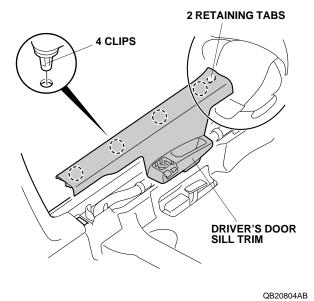
2-Door: Two retaining tabs and six clips.
