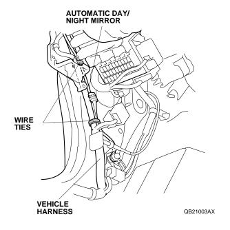
32. Route the automatic day/night mirror harness upward. Secure the automatic day/night mirror harness to the dashboard with one wire tie as shown.
