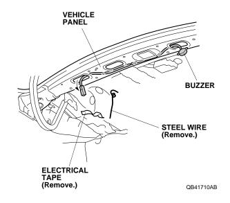
23. Using isopropyl alcohol on a shop towel, thoroughly clean the vehicle panel where the buzzer will attach.
