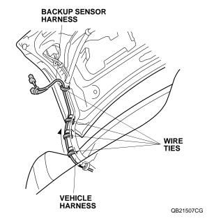
33. Unplug the vehicle 2-pin connector (Green) from the left taillight, and plug it to the backup sensor harness 2-pin connector.
