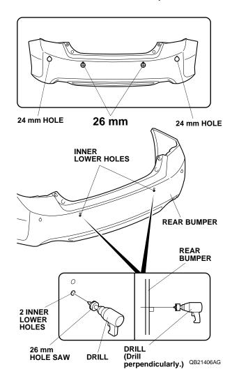
12. Using the sensor clips, install the two center sensors (Blue) into the 26 mm holes in the rear bumper. Note the direction and the pin location for each sensor.
