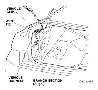
Align the green tape on the backup sensor harness with the vehicle clip, and secure the backup sensor harness to the vehicle harness with one wire tie as shown.
