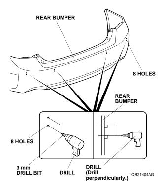
Using a 24 mm hole saw, enlarge the outboard (left and right corner sensor) bumper holes by drilling the lower 3 mm holes. Remove any burrs.
