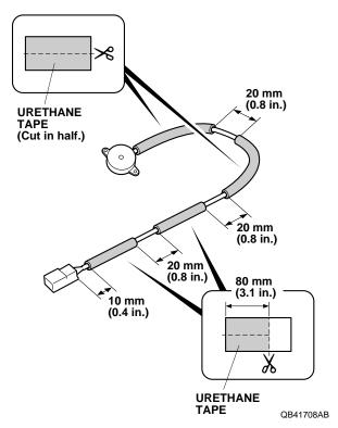
19. Using scissors, cut one urethane tape into three pieces. Wrap the two 80 mm cut pieces of urethane tape around the buzzer harness at the measurements shown.
