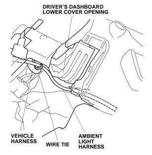
19. On the passenger's side of the vehicle, route and secure the ambient light harness to the vehicle harness with one wire tie.
