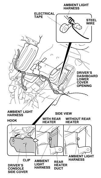
14. Attach a piece of steel wire to the ambient light harness with electrical tape. Route the ambient light harness through the center console from the driver's dashboard lower cover opening to the passenger's under cover opening.
