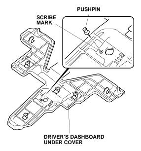
22. While wearing eye protection, drill the pierced mark on the driver's dashboard under cover with a 3 mm drill bit, then enlarge the hole to 5 mm using a 5 mm drill bit. Remove all burrs.
