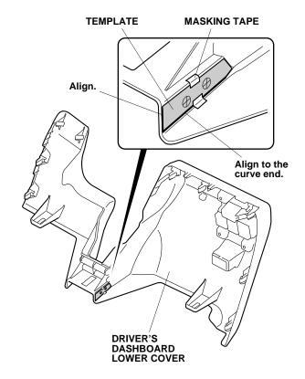
27. Using a pushpin, pierce the center of the two marks on the template.
