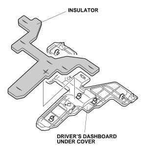
21. Using a pushpin, pierce the center of the scribe mark on the driver's dashboard under cover in the area shown.
