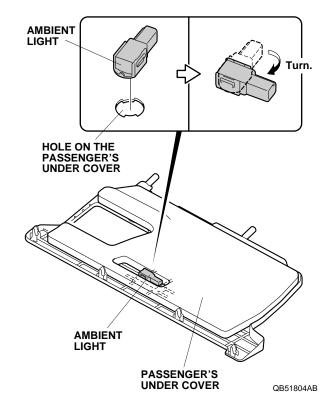
24. Plug the ambient light harness 2-pin connector into the ambient light, and reinstall the passenger's under cover.
