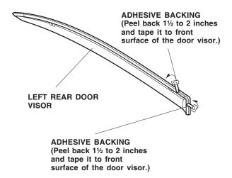
13. Align the hole in the visor with the mark you made on the masking tape, and install the clips.
