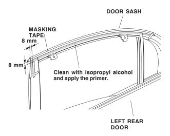
11. When the isopropyl alcohol is dry, carefully apply primer to the door sash. Wipe off any excess primer immediately. Allow the primer to dry for at least 3 minutes.
