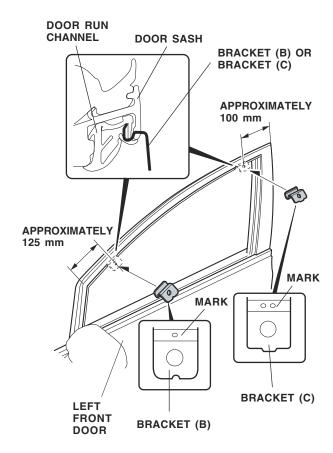
19. Install a bracket (B) and a bracket (C) on the door sash at the measurements shown. Verify the shape and the identification mark stamped on each bracket. Be sure to use the correct bracket at the proper location.
