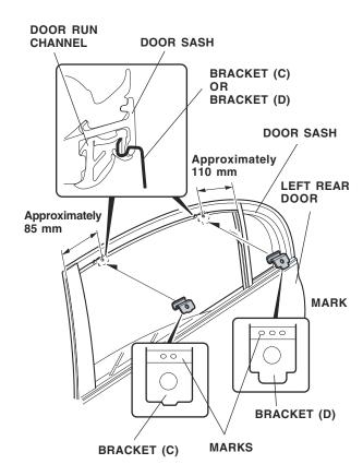
2. Install a bracket (C) and a bracket (D) on the door sash at the measurements shown. Verify the shape and the identification mark stamped on each bracket. Be sure to use the correct bracket at the proper location.
