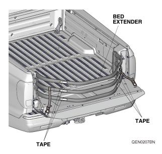
Adjust the bed extender width installed in the vehicle and secure them with tape. Make sure it can pivot and be uninstalled without much effort.
