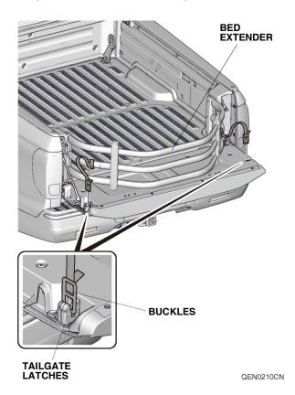
15. Release the buckles by pulling the tailgate handle. Unlock the rear latches by pulling the lever toward you and remove the bed extender by lifting it upward.
