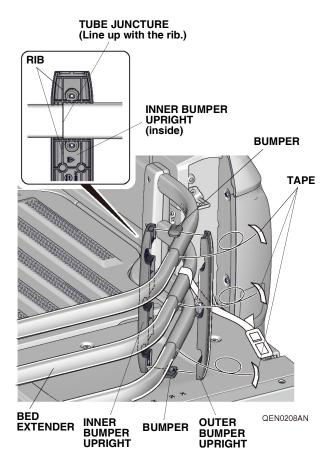
12. Secure the bumper uprights to the bed extender with six PT-screws in the order shown. Tighten the PT-screws evenly.
