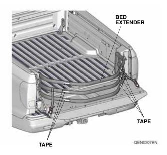
Adjust the bed extender width installed in the vehicle and secure them with tape. Make sure it can pivot and be uninstalled without much effort.
