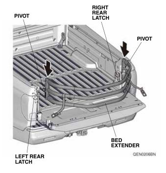
9. Carefully pull down the bed extender onto the tailgate.
