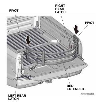
19. Rotate the bed extender forward. Close the tailgate.
