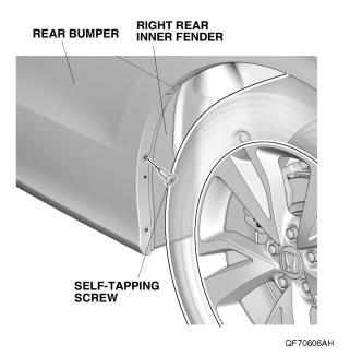
16. Install one spring nut into the right rear inner fender hole. NOTE: Make sure to install the spring nut in the
