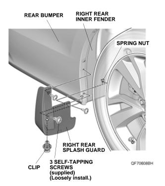
18. Secure the right rear splash guard with the three self-tapping screws in the order shown below. NOTE: Make sure there is no gap between the right rear splash guard and the bumper. If there is a gap, loosen the self-tapping screws, hold the splash guard against the bumper, and retighten the screws.
