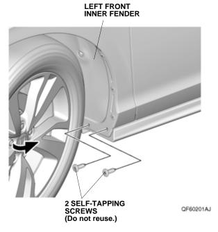
2. Remove the two self-tapping screws from the left front inner fender.
