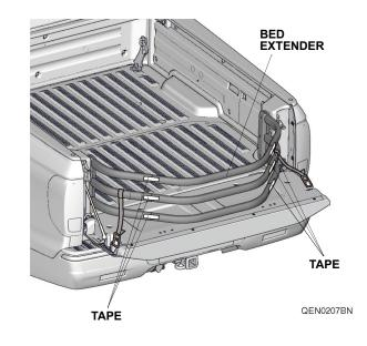
10. Adjust the bed extender width installed in the vehicle and secure them with tape. Make sure it can pivot and be uninstalled without much effort.
