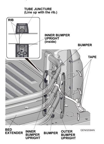
12. Secure the bumper uprights to the bed extender with six PT-screws in the order shown. Tighten the PT-screws evenly.
