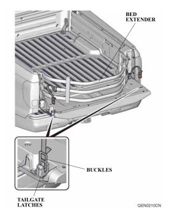
15. Release the buckles by pulling the tailgate handle. Unlock the rear latches by pulling the lever toward you and remove the bed extender by lifting it upward.
