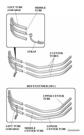
7. Install the strap to the middle tube of the right tube. Slide three center tubes into the right tube using the coated area as a guide for depth of insertion.
