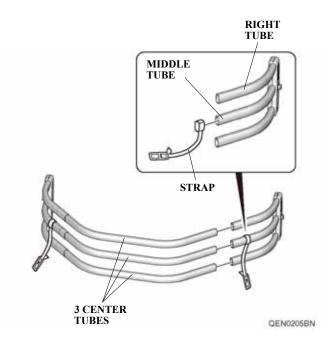
8. Insert the two pivots on the bed extender into the rear latches. Push down on the bed extender until the parts are locked.
