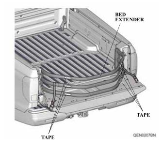
10. Adjust the bed extender width installed in the vehicle and secure them with tape. Make sure it can pivot and be uninstalled without much effort.
