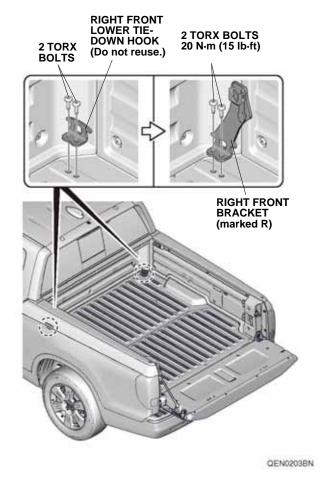
5. Install the right front bracket with two TORX bolts removed in step 4. Torque the TORX bolts to 20 N·m (15 lb·ft). Repeat steps 4 and 5 on the other side.
