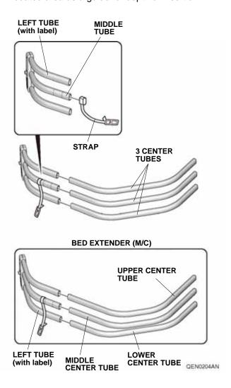
7. Install the strap to the middle tube of the right tube. Slide three center tubes into the right tube using the coated area as a guide for depth of insertion.
